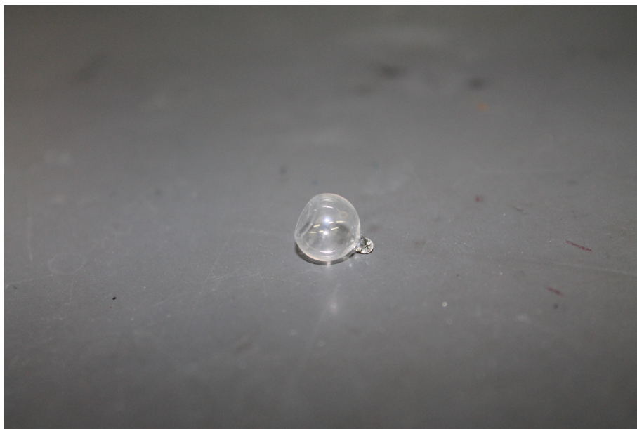
Figure 4.1: This is the cell used for the majority of experiments in this thesis. Its Ehrenmeyer flask like shape caused the laser beams to be greatly distorted.
