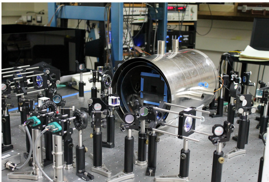
Figure 6.1: The apparatus is shown within the shields. Note the asymmetry of the ports in the shield; this forces us to place the cell and field coil setup closer to one endcap than the other, which is a main cause of field gradients. The pulsing field coils have been designed to minimize these gradients.
