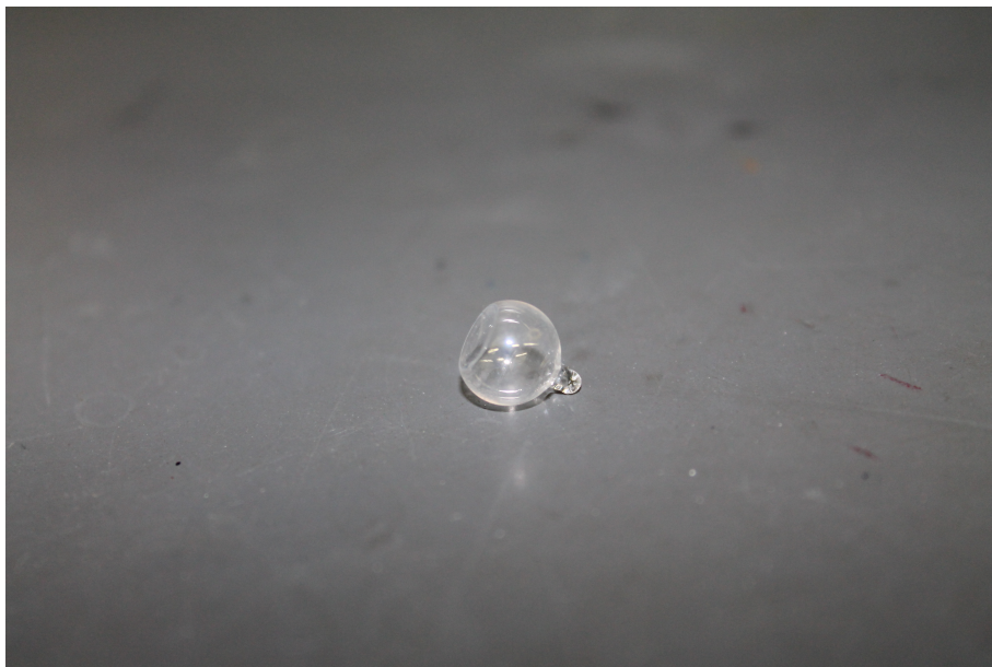
Figure 6.2: This is the cell used for the majority of experiments in this thesis. Its Erlenmeyer flask like shape caused the beams to be greatly distorted.
