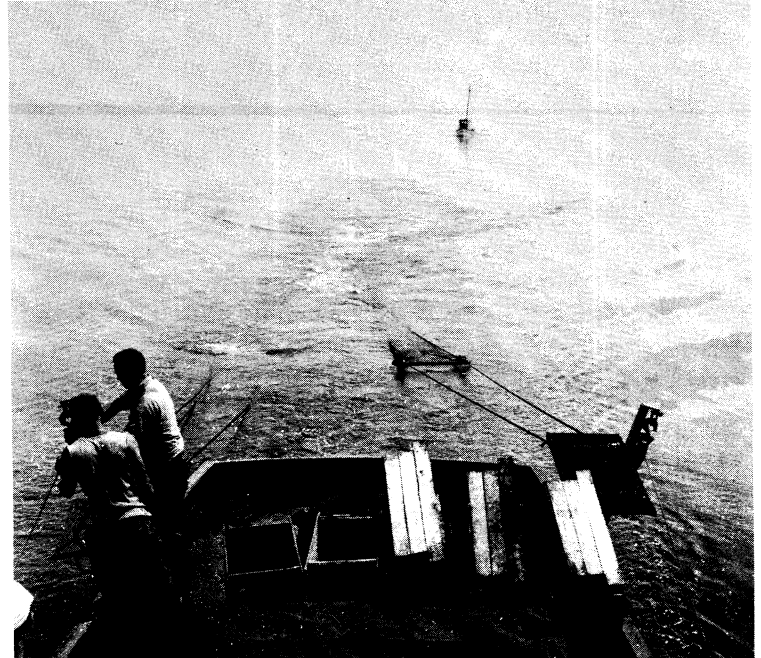
Releasing the trawl to continue fishing. Otter boards keep the trawl on the bottom and spread the trawl out.
