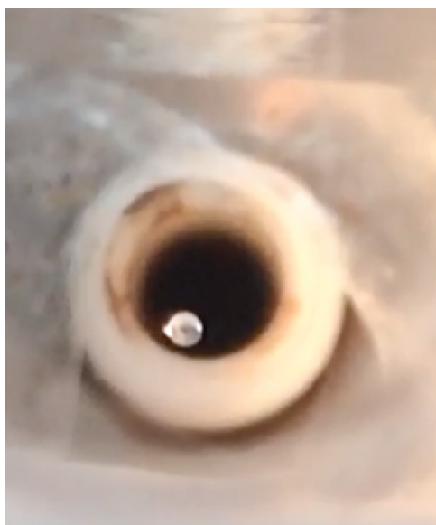
Figure 4.5 A droplet about 0.8 mm in diameter levitated in the acoustic levitator. The round object in the back is a homemade inlet extension of a mass spectrometer.
