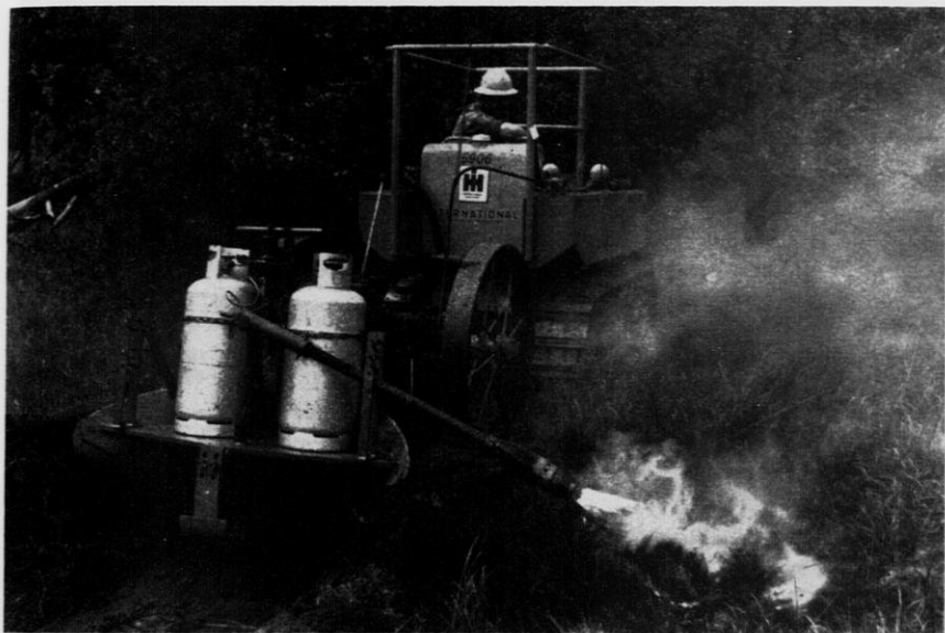
Here a tractor-tanker is equipped with an automatic backfiring device which the Conservation Department developed.
