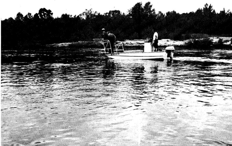
*A.C. boom shocker used to stun and capture lake sturgeon. Note the large nets.*
