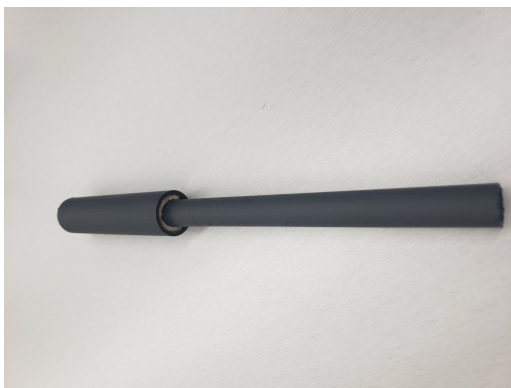
(a) Two tubes connected with a HDF ring
