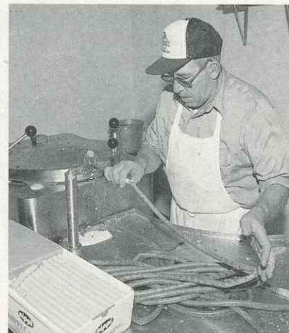
(right) Commercial sausage-makers follow the same steps on a larger scale. Here "hot sticks" are formed in an electric stuffer controlled with a foot pedal.
