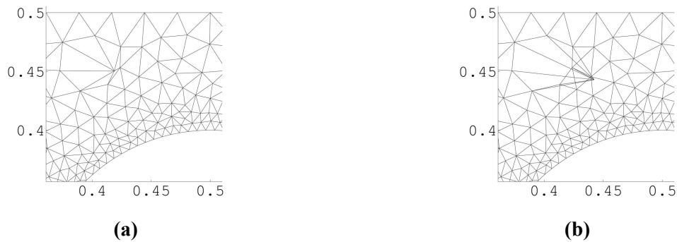
Figure 64: (a) A mesh with a poor quality element that is subsequently fixed by (b) moving the node to a new position where the mesh happens to be tangled.
