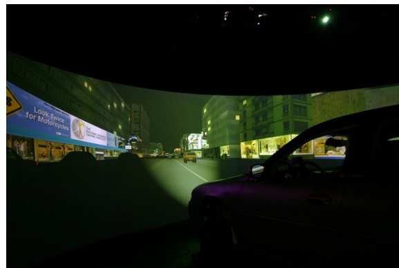
Figure 10 Illustration of a projected driving environment on the inside of the dome. Reprinted from Brown et al. (2011).
