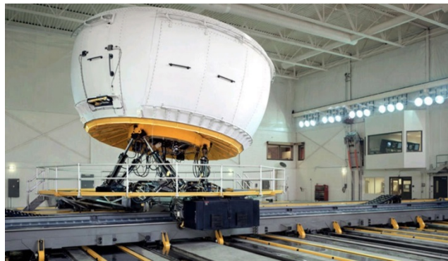
Figure 9 Dome and motion base structure of the NADS II simulator. Reprinted from Brown et al. (2011).
