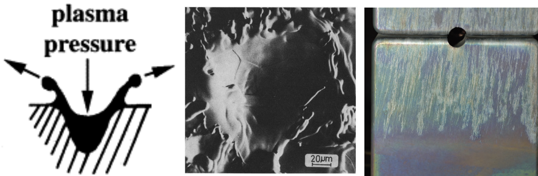
Figure 2.8: At left, a depiction of cathode spot erosion of a cathode surface, from [3]. Middle, from [4], a cathode spot crater in an arc track on a tungsten cathode. Right, from [5, 6, 7], cathode spot tracks on the upper divertor of ASDEX-U.
