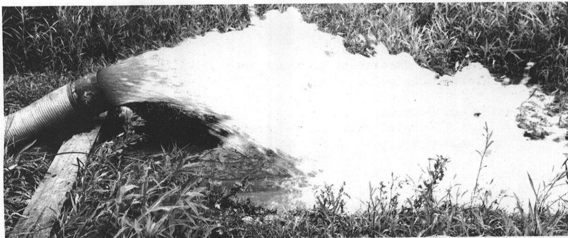
Water discharging from the 6-inch discharge tube of an outboard pump.
