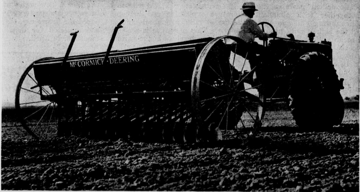
Above: Drilling moves along fast with a McCormick-Deering Grain Drill and Farmall 20 Tractor on the job. Right: A good job of disking and harrowing. The disk is an 8-foot McCormick-Deering with a 2-section McCormick-Deering Peg-Tooth Harrow pulled behind.
