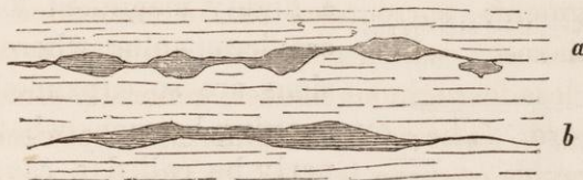
a. Crevice with pocket openings. b. Crevice opening.
