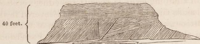
FIG. 8.—Section on Legate Branch, exhibiting Cross-stratification of the Upper Sandstone.
