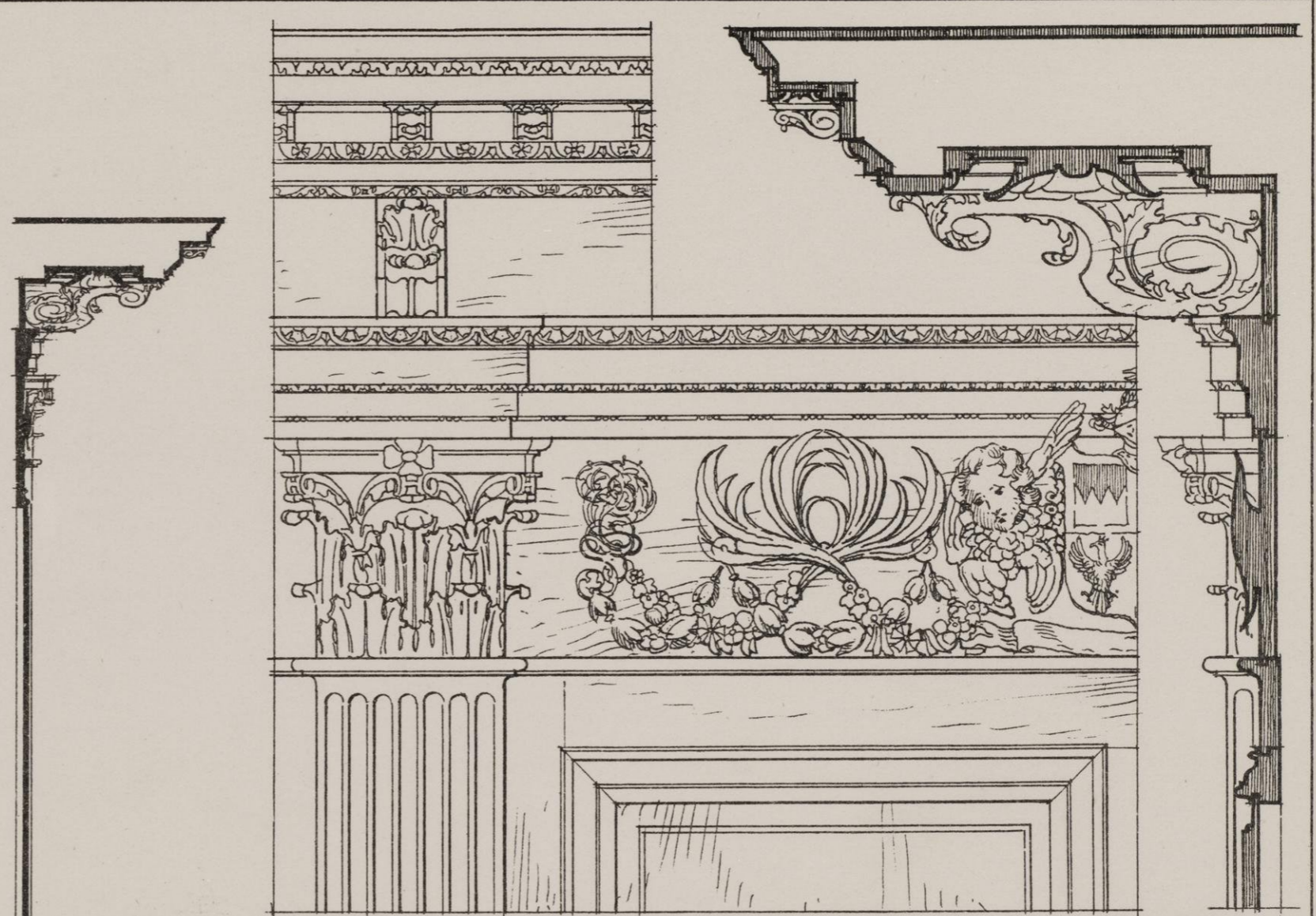
ELEVATION OF FRIEZE AND CORNICE (DETAIL)
