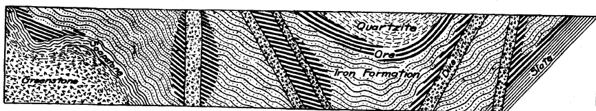
Fig. 37. Marquette Range. Ideal cross section showing various ways in which ore occurs.
