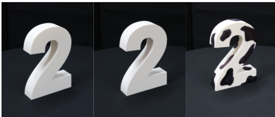
Figure 6.8: “2” objects with different reflectance properties used in the varying scene reflectance experiment (Sec. 6.7. From left to right: matte white, glossy white, and spotted black and white.
