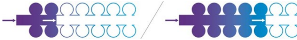
Figure 7.3: Analogy of water flowing through a pipe with “pockets” to explain charging currents in cable-based transmission, from [46]
