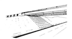
SLOPE PAVING UNDER STRUCTURES
