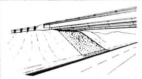
SLOPE PAVING UNDER STRUCTURES
