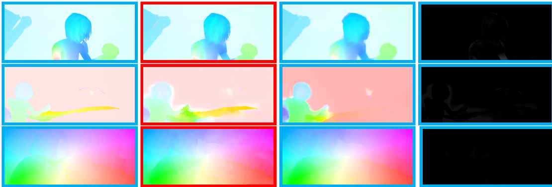
Figure 3.1: Optical flow results on the MPI Sintel dataset. Columns 1 to 3 (5 to 7) show the ground truth, our result and the Epicflow result respectively. Column 4 shows the error map. AEE's of column 4 are 1.08, 1.15, 1.03 for rows 1 to 3. Our results are marked in red.
