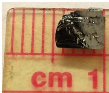
**Figure 6.1.** A photograph of a large flux-grown crystal of  $\text{ScCoGa}_5$ .
