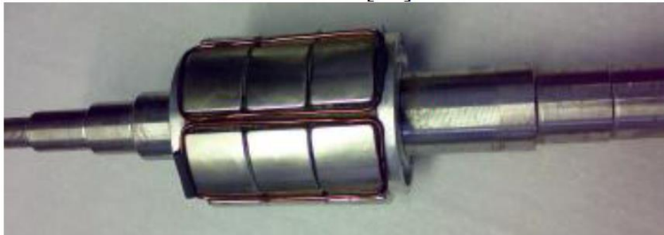
Fig. 1-19 SPMSM rotor design with short-circuited copper ring [51]
