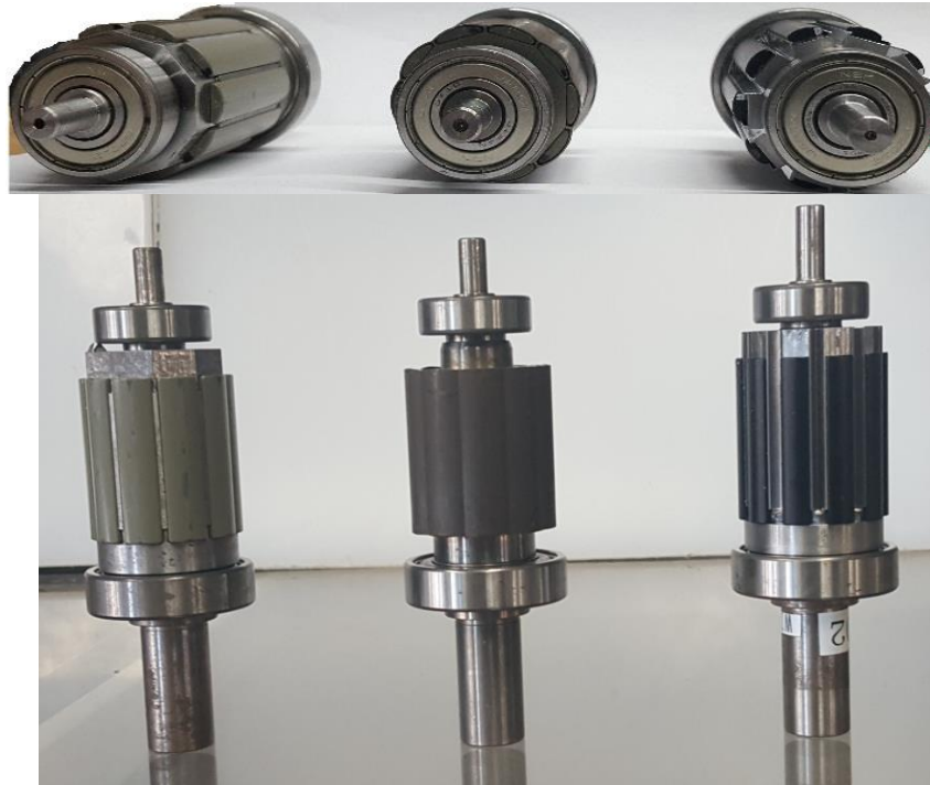
Fig. 2-47 The fabricated rotors (left) SPMSM (center) IPMSM (right)FI-SPMSM
