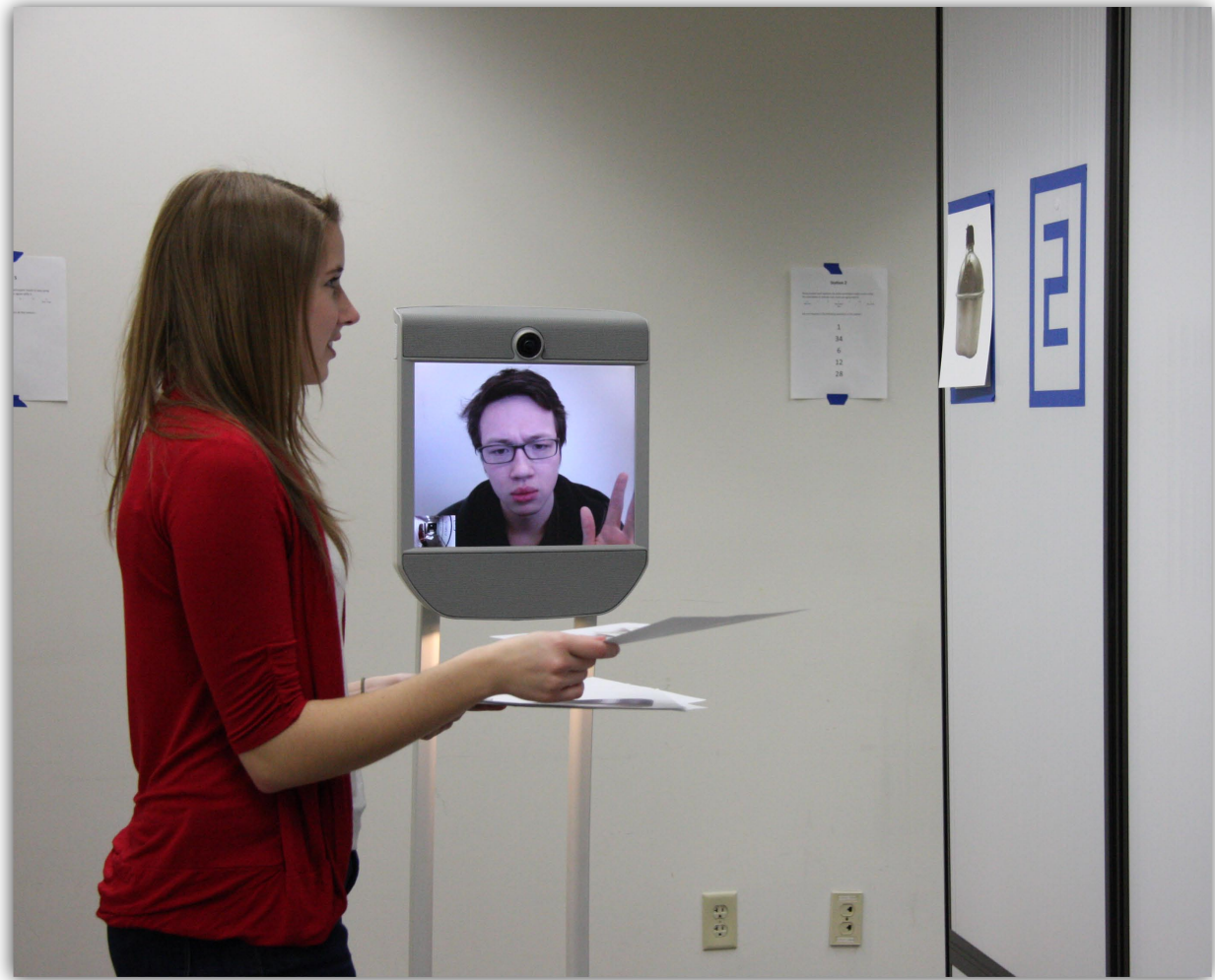
Figure 6.1: “Local” participant interacting with a “remote” confederate via a Beam telepresence robot.
