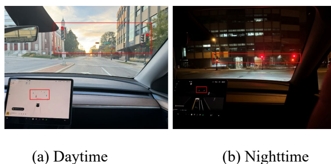
Figure 3.10. Illustrations of Tesla traffic light testing during the daytime and nighttime.
