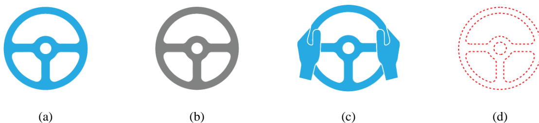
Figure 8. Dashboard graphics for automation status. (a) On, (b) Off but available, (c) Takeover request, and (d) Off and unavailable.
