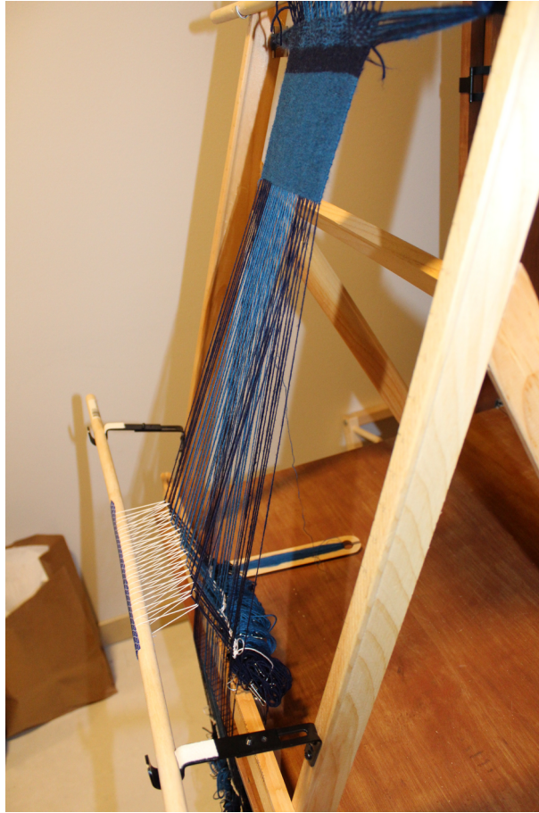
Figure 8: Side-view of warp-weighted loom demonstrating the open shed from experimental archaeological study by author, wood, wool. Image by Morgan Lemmer-Webber, Creative Commons Attribution-Share Alike 4.0 International.
