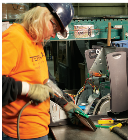
Data security procedures at Universal Recycling Technologies in Janesville include drilling holes in a computer hard drive.
