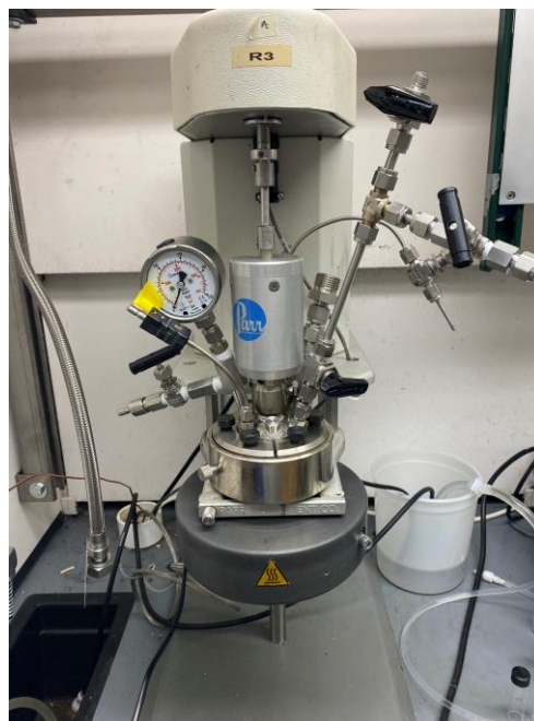
Figure A 5.1. Picture of top part of autoclave reactor (left) showing Teflon stirrer, thermocouple, and optional Teflon sampling/dip tube with pinhole sampling port. Right picture shows autoclave reactor mounted in heating mantle. The top attachments include pressure gauge with gas addition/removal quick connect needle valve, thermocouple plug, catalyst addition (under pressure) valving, sampling (under pressure) tube, and stirrer magnet going counterclockwise from the left. For ambient pressure experiments the catalyst addition valving is replaced by a 11 mm septum fitted into 1/2" tubing connected via SwageLok fittings.
