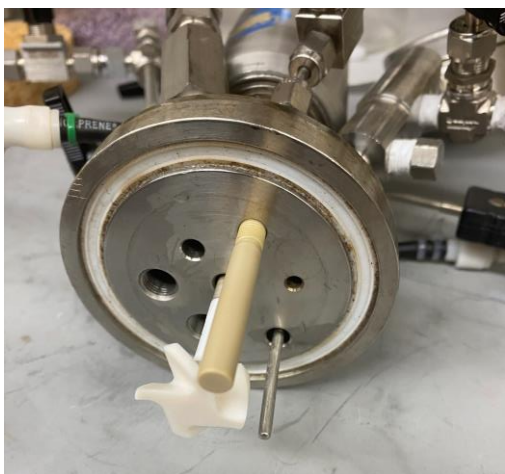
Figure A 5.1. Picture of top part of autoclave reactor (left) showing Teflon stirrer, thermocouple, and optional Teflon sampling/dip tube with pinhole sampling port. Right picture shows autoclave reactor mounted in heating mantle. The top attachments include pressure gauge with gas addition/removal quick connect needle valve, thermocouple plug, catalyst addition (under pressure) valving, sampling (under pressure) tube, and stirrer magnet going counterclockwise from the left. For ambient pressure experiments the catalyst addition valving is replaced by a 11 mm septum fitted into 1/2" tubing connected via SwageLok fittings.
