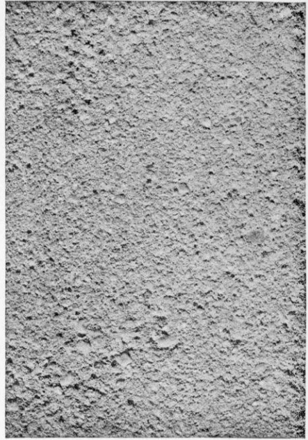
YELLOW BAR SAND AND CEMENT, COMPOSED OF ONE PART CEMENT AND THREE PARTS YELLOW BAR SAND
