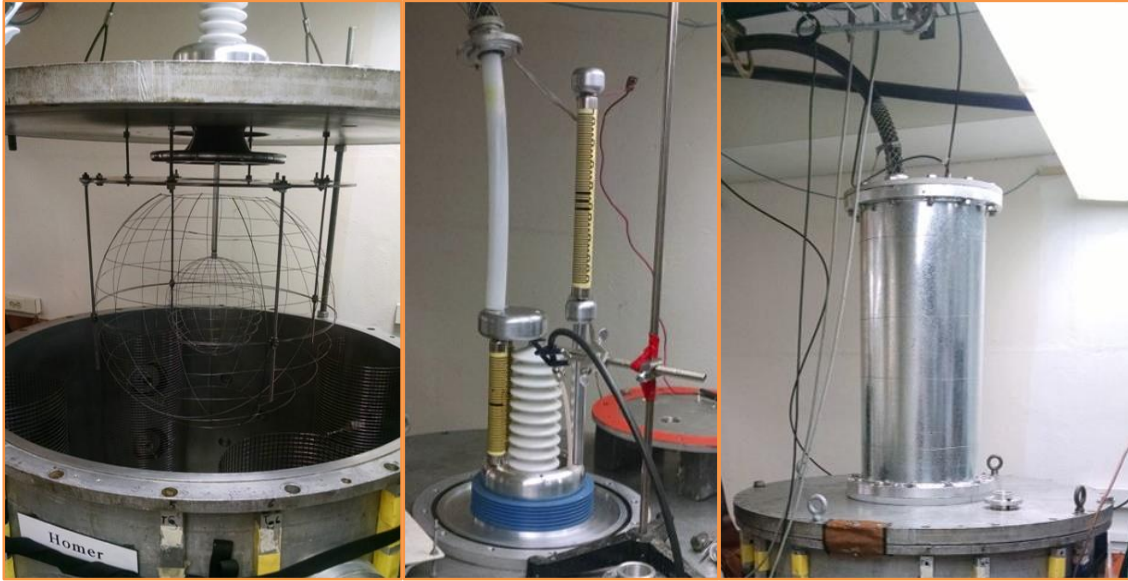
Figure 4-10: Assembly of the grids and shield electrodes (left), in air testing of the voltage divider circuit (center), full feedthrough assembly with dielectric oil tank (right).
