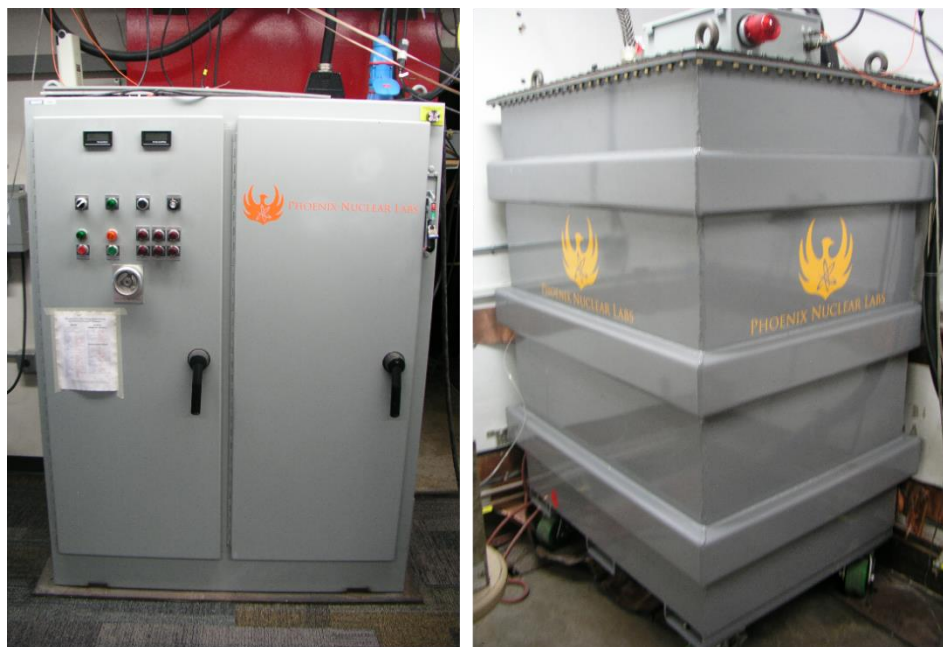
Figure 4-2: Negative Polarity 300 kV DC high voltage power supply control (left) and high voltage tank (right) used for this work; manufactured for the laboratory by Phoenix, LLC.
