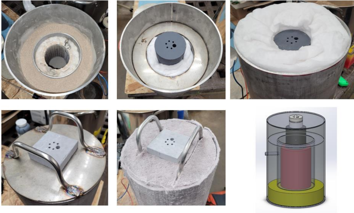
Figure 23: Model and fabrication photos of the custom-built calibration furnace.
