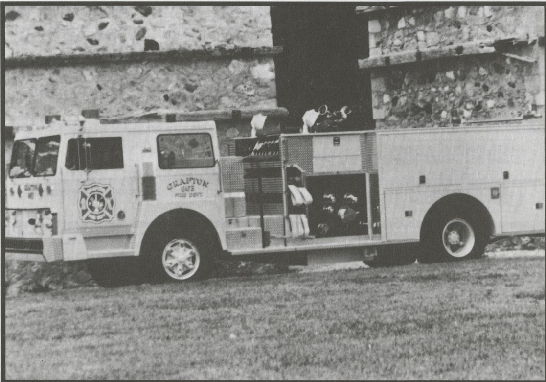
This 1978 Pierce 1,500 GPM pumper featured a top-mounted pump panel. One of the first of its kind, it was copied by the New York City Fire Department.
