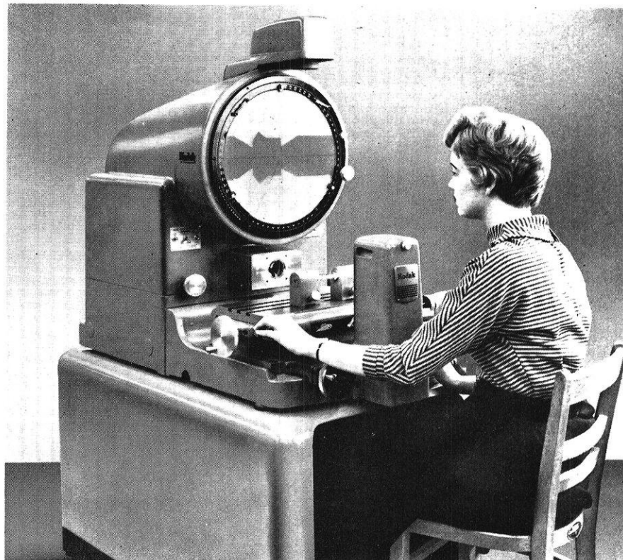
Embodying a micrometer device for horizontal measurements, the new Kodak Contour Projector, Model 14-6 features ample table travel to simplify staging. The projector, which will be shown for the first time at the Western Metal Exposition, March 25-29, in Los Angeles, is expected to find wide application in receiving-inspection and tool-room optical gaging.
