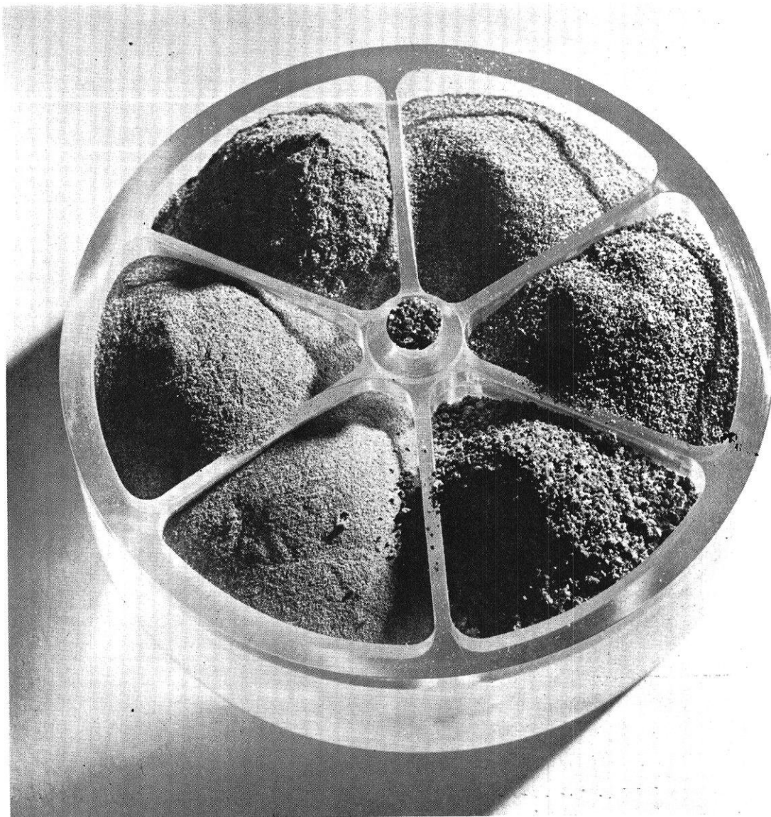
In the photo above, the man-made diamonds are separated into grades according to usual industrial classifications. The plastic container is approximately three and one-half inches in diameter.
