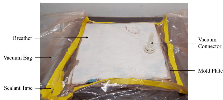
Figure 5.4: Laminate manufacturing setup
