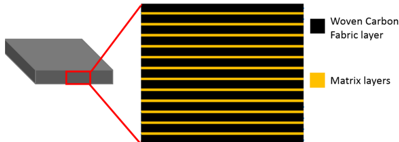
Figure 4.2: Schematic of fabric layers and interlaminar regions of the laminate
