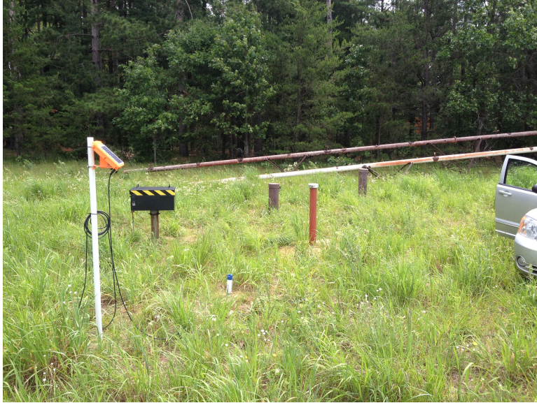
Figure 5. Installation in the Prairie. In addition to the four groundwater monitoring wells and piezometers, a soil moisture probe (shown in the foreground) and a weather station (not shown) have also been installed.
