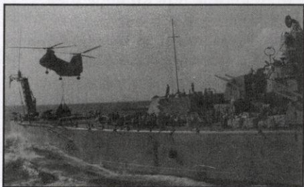
Both the Mars and the Niagara Falls would transport stores ship to ship by helicopter.
