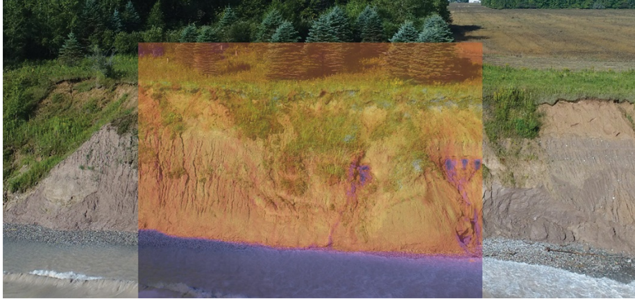
Figure 8. Thermal image overlaid on optical image showing discrete areas of groundwater discharge. These seeps (shown as dark blue) are 12-23°F colder than the surrounding bluffs but were not visible in the optical imagery due to obscuration by vegetation.
