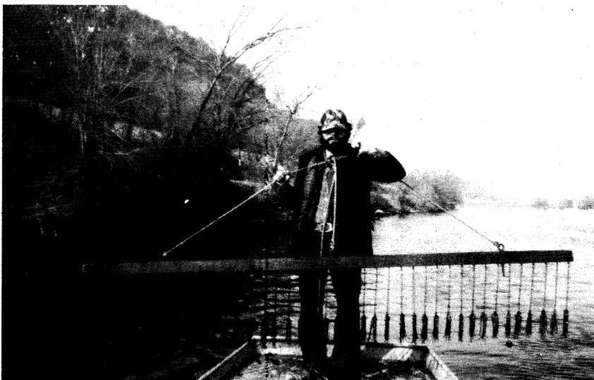
The 10 ft brail, equipped with 200 dovetail hooks, that was used during the study.
