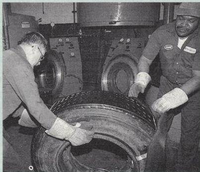
In the mold method of retreading (top three photos) a thick layer of rubber is wrapped around a tire casing. The prepared casing is set in a tread mold, heated and pressed. Rubber nibs are trimmed and recycled after the fresh retread cools. (bottom photo) Using the precure method, a casing is buffed and preformed tread is bonded and vulcanized to the tire. Photos by Robert Queen
