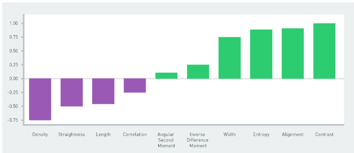
Figure 2.5: Coefficient weights assigned to each attribute in an SVM classification model. Negative values are of equal importance to classification as positive.
