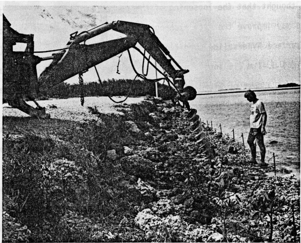
Figure 4. Power auger used to bore transplant holes (Site C).
