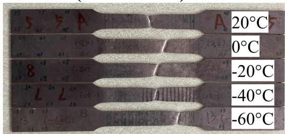
Figure 4.5: The failure modes of the specimens at fracture. Necking is observed in DP-580 and Mild-395 specimens.
