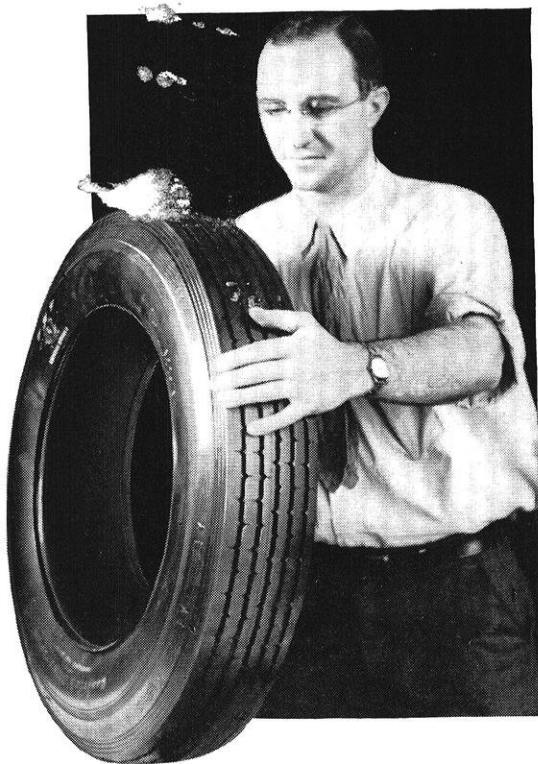
Inspecting an "Ameripol" tire, which is identical in appearance to a natural rubber casing.
