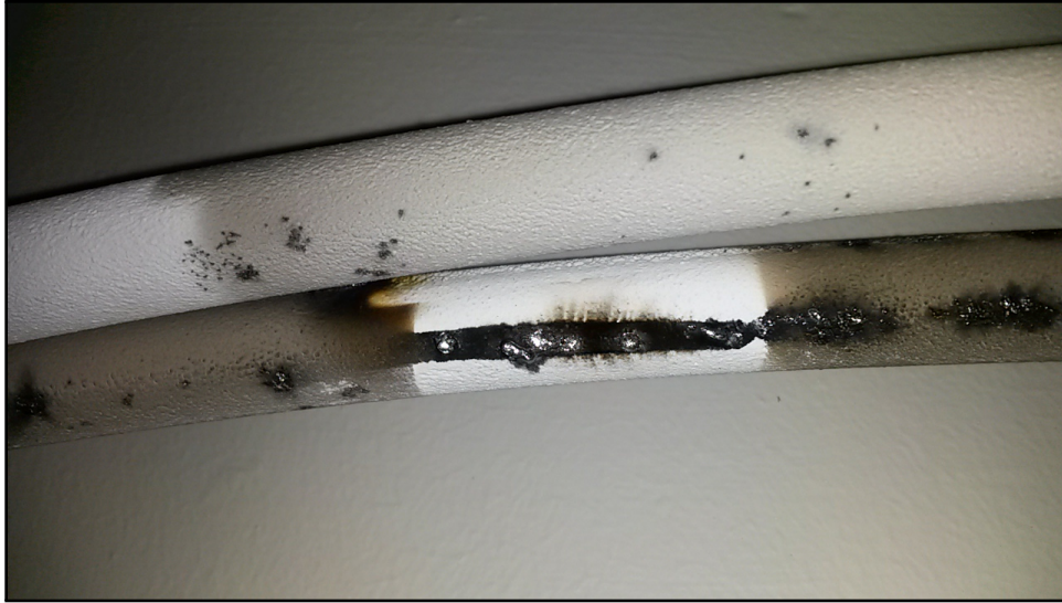
Figure 5.1: An image of the alumina insulating material after the experimental campaign from Chapters 3 and 4. A support clamp held the coil where the alumina is brightest in color with the lighter discoloration coming from general plasma exposure. The metallic spots are sputtered aluminum, surrounded by what appears to be burnt alumina.
