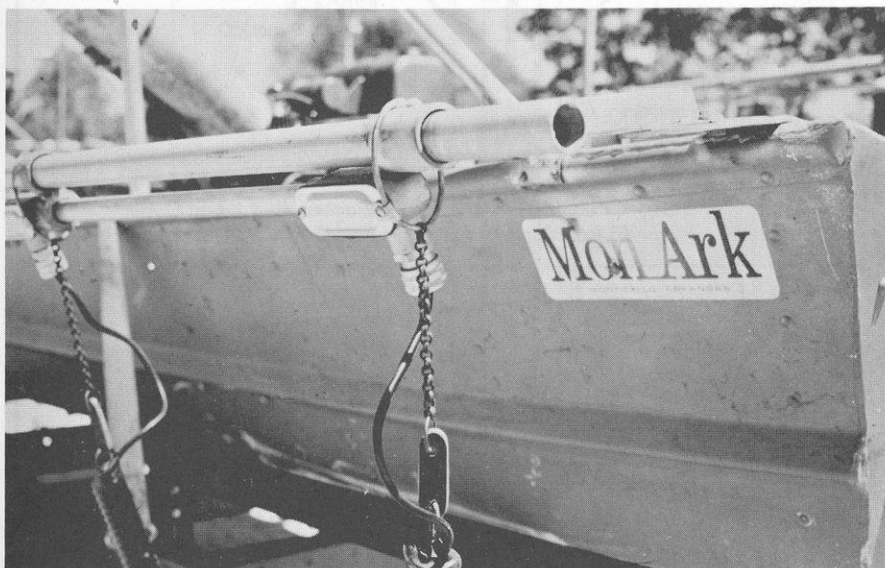
Cathode array support and power supply system.
