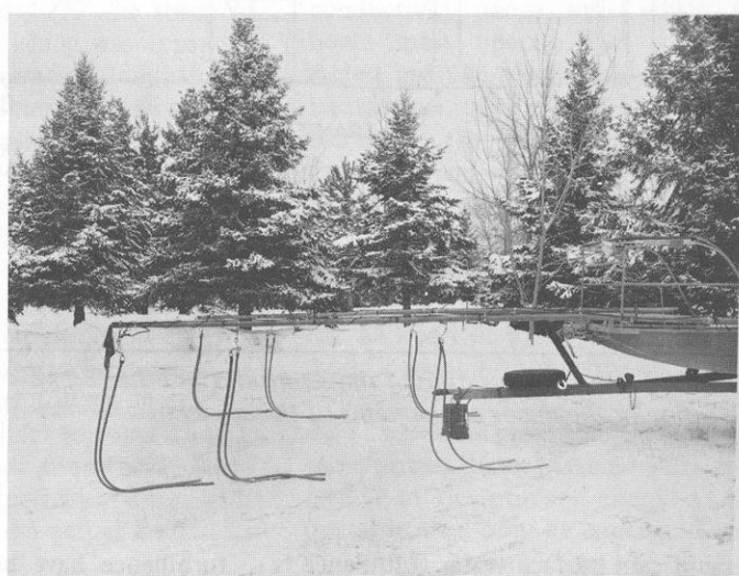
Alternate polarity electrode array (Top). Multiple pair electrode array (Bottom).
