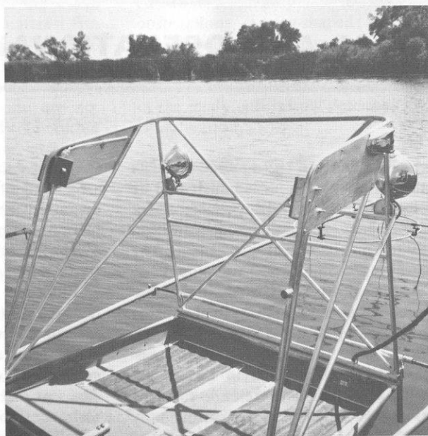
Floor mat switches are permanently installed on the front deck. Safety railing surrounding the front deck to protect operators and support main lighting system, bow running lights and the safety on-off controls. The boom support structure for adjusting height and spacing is fastened to the bow.
