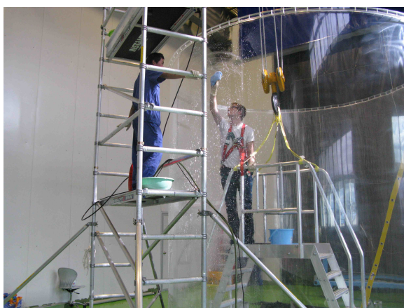
(a) Scrubbing the OAV inside with 1% Alconox solution.
