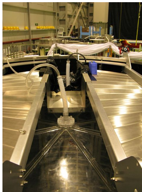
(b) Photograph of the IAV tube stack leak-checking setup. An argon sniffer is run up and down the tube stack, which is pressurized with argon gas.
