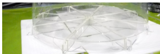
(d) Image of a fabricated IAV bottom during cleaning. Notice that all structural support is located on the IAV outside.
