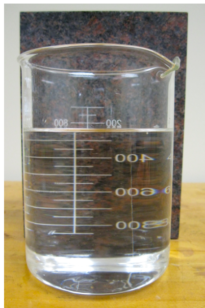
(b) Acrylic sample polished to 400-grit, immersed in mineral oil.
