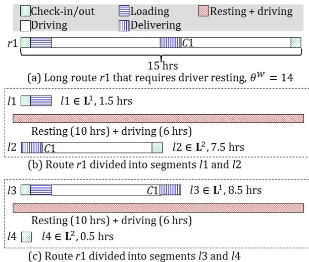
**Figure 3.6.** All ways to break long routes into segments are considered.
