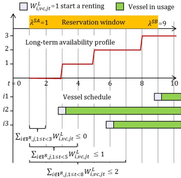
**Figure 4.6.** Constraining the number of unreserved vessels in long-term mode according to the availability profile.
