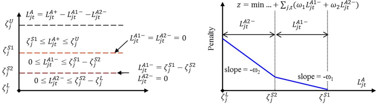
**Figure 2.7.** Piecewise linear penalties for inventory below  $\zeta_j^{S1}$  and  $\zeta_j^{S2}$ .
