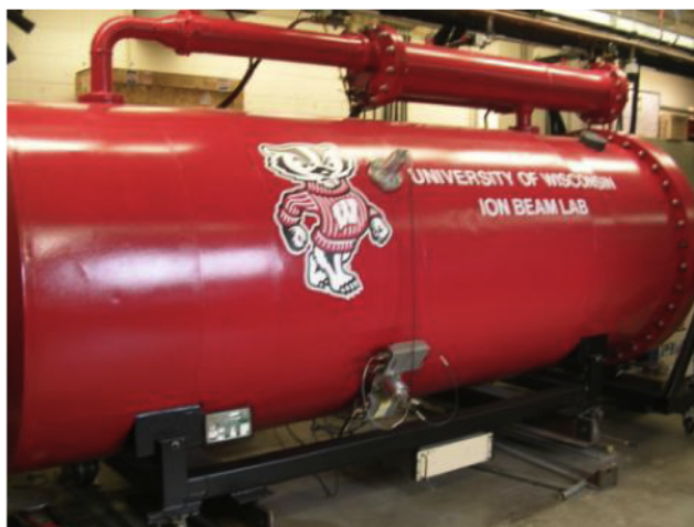
Figure 31: University of Wisconsin – Madison Ion Accelerator that was used to perform 2.6 MeV H^+ and 3.9 MeV He^{2+} irradiations.
