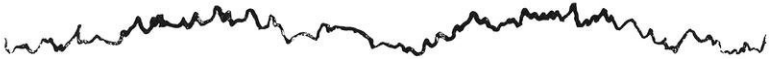
FIG. 4.—Standard De Laval; engine loaded to about one-half of its greatest capacity Horse power per card, 1,619.
