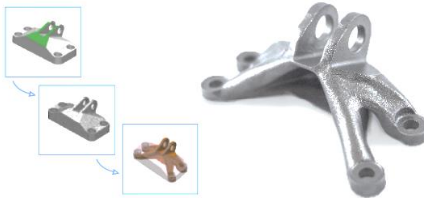
Figure 83: An example of 3D printed structures designed by topology optimization
