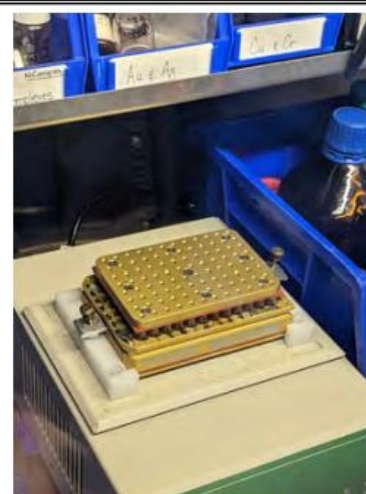
Image 5. Heating/shaking the block assembly in a glovebox for 36 hours.
